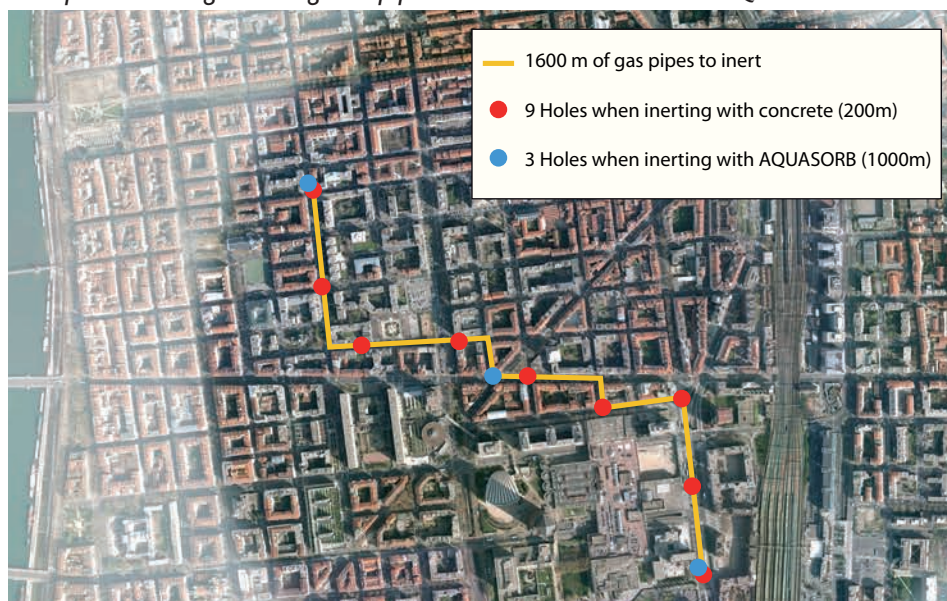
Example of inerting on a length of pipe of 1600 m without or with AQUASORB
